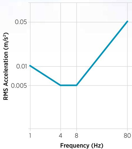
**Fig. 2:** The ISO Base Curve (isoperceptibility line) for human perception of vibrations along the axis of the spine is the basis for most serviceability criteria.
