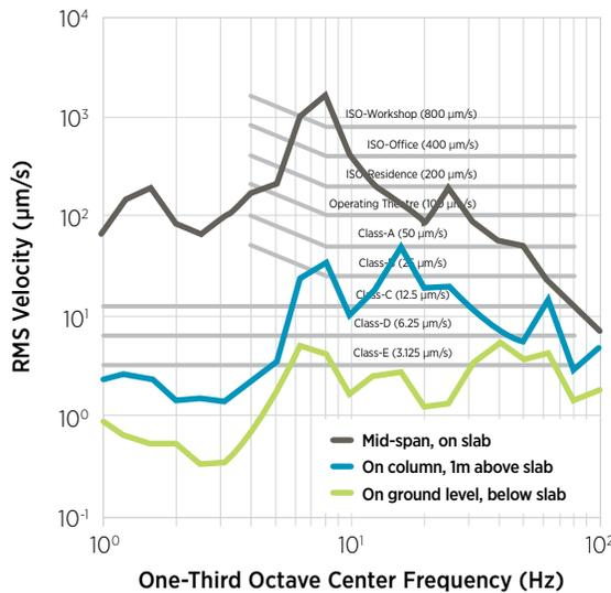
**Fig. 8:** Vibration responses due to a ½ ton pickup travelling at 15 mph over an expansion joint on the second level of a parking garage. The garage is located above an ambulatory surgical clinic at ground level. Through analysis of concurrent measurements of slab motions, support column motions and vibration levels on ground level below, these data were used to design secondary/isolated structural framework to control vibration transmission to operating rooms and patient care areas.
