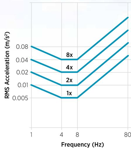
**Fig. 3:** Multiples of the ISO Base Curve (e.g., 2x, 4x, etc.) are specified for occupied spaces where human comfort is a concern. Increasing multiples indicate reduced sensitivity to structural motions.
