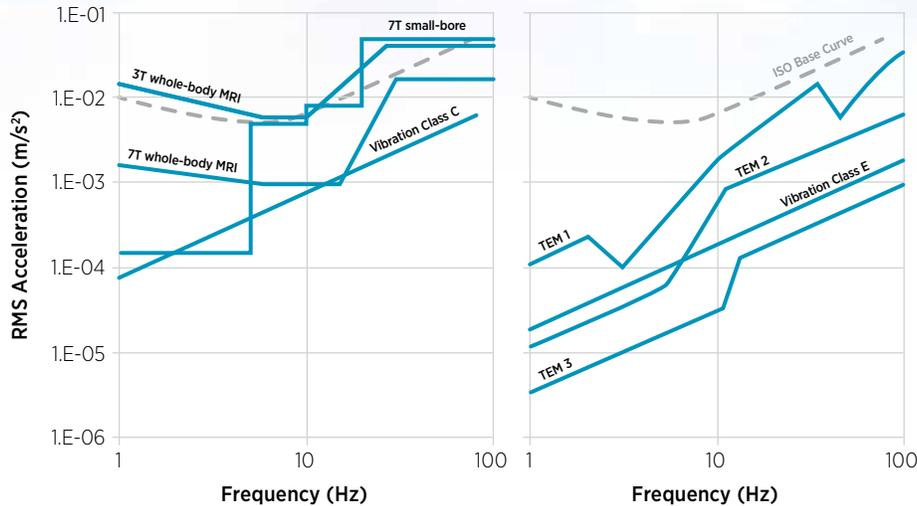
**Fig. 5:** Examples of vendor criteria for various medical imaging (left) and high resolution microscopy devices (right). Data is shown in units of RMS acceleration for direct comparison of different types of equipment. Also shown are the ISO Base Curve (threshold of human perception, head-to-toe direction), and vibration classes C and E for reference. When available, vendor criteria should always be used as a basis for assessment.
