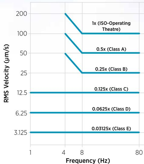
**Fig. 4:** Fractions of the ISO Base Curve [e.g., 0.5x, 0.25x, etc.] are specified for occupied spaces where sensitive equipment, animals and procedures are a concern. The ISO-Operating Theatre curve is equivalent to the ISO Base Curve (from which generic serviceability specifications are derived). Varying multiples/fractions of the base curve are specified according to the use and occupancy of the space.
