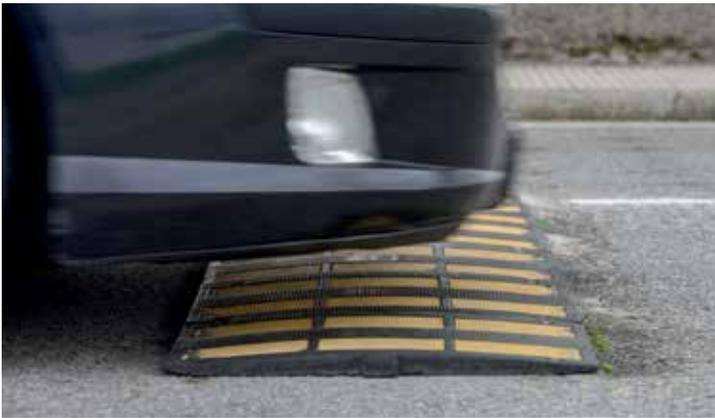
**Fig. 6:** Traffic calming measures such as speed bumps can be useful for controlling speeds in some areas. However, such obstructions should have broad, shallow slopes to reduce the vehicle forces imparted to the structure.
