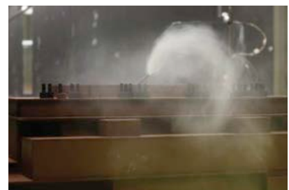
Exhaust emissions on building rooftops are often directed downward by local wind flow patterns.
